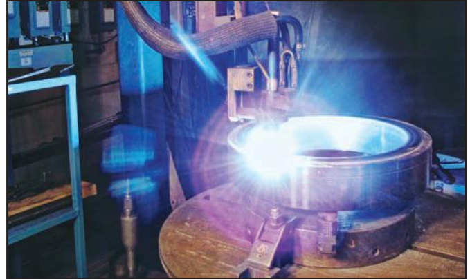
Automatic plasma arc hardfacing equipment for seats.
