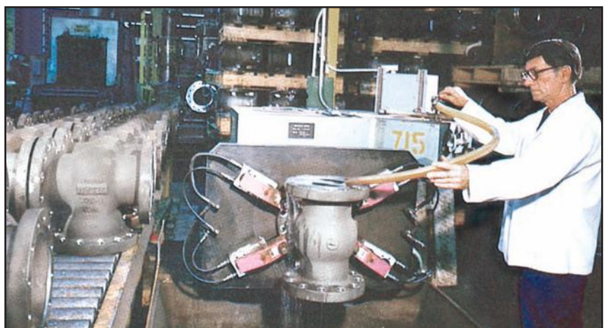
2 Air-under-water test of the seat's welds.
