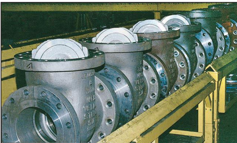
7 Assigning the ideally fitted wedge, ground and lapped, to its proper valve body.
