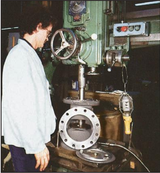
3 Relapping of seating faces after seal welding.
