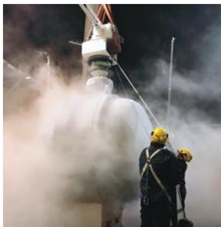
A Vanessa 96" double flanged cryogenic valve tested at Lugagnano plant (Italy).
