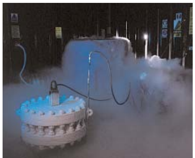
Cryogenic test facility for helium leak testing
