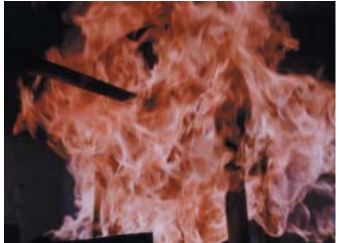
16" 600 lb BFR Flanged Check Valve undergoing firetest
