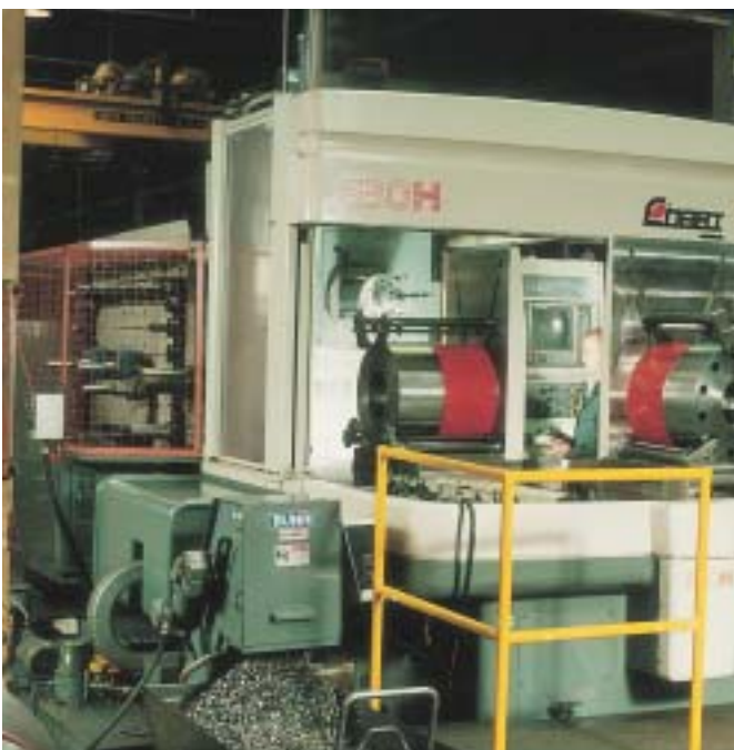
Twin Pallet CNC machining centre with 60 tool changer
