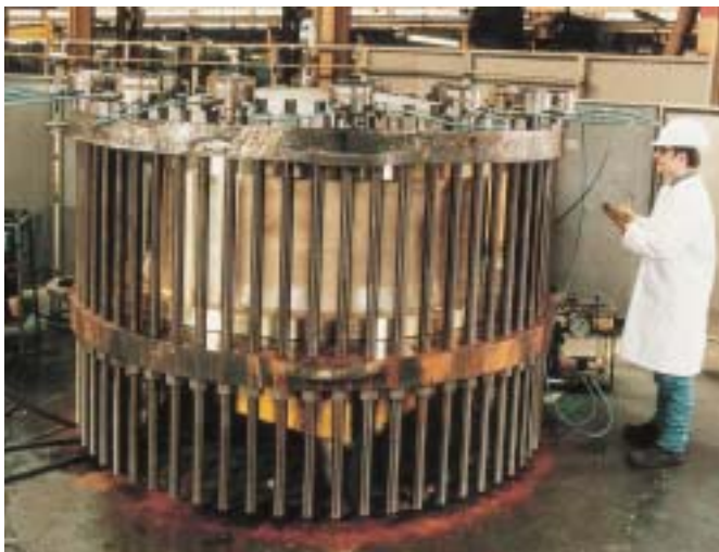
84" 150 lb valve undergoing hydrotest in Goodwin factory
