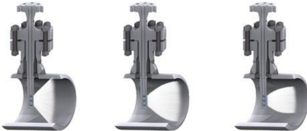
Figure 7.3 Desuperheater Spray Penetration
