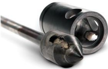
Figure 5.9 Typical Appearance of Cavitation Damage
