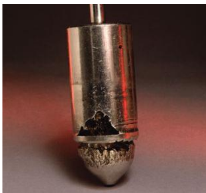
Figure 5.8 Typical Appearance of Flashing Damage
