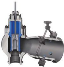
Figure 7.10 Cross-Section View of Steam Conditioning Valve
