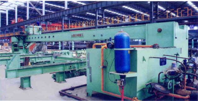
▶ 水压机1 Hydrostatic test machine
