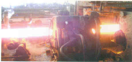
▶ \Phi 76 穿孔机 Piercing mill
