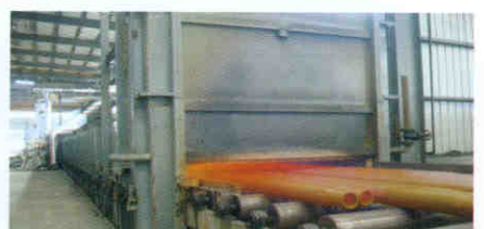
▶ \Phi 219 热处理炉 Heating furnace
