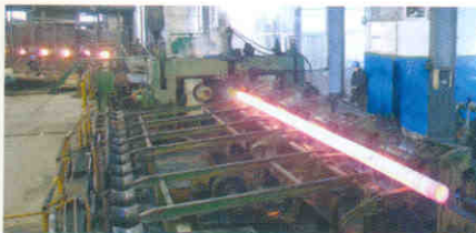
▶ \Phi 219 穿孔机 Piercing mill
