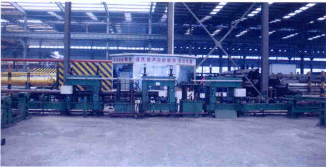
▶ 超声涡流联合探伤机组 Joint Inspection Unit of ultrasonic eddy current
