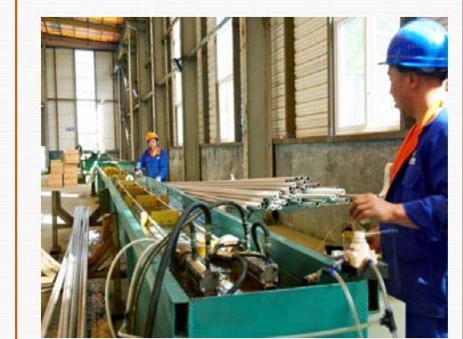
Air Pressure Test
