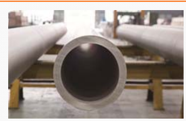
Hydrogenation Furnace tube
