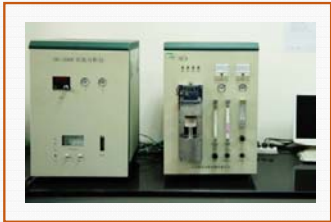
NCS Oxygen -Nitrogen Analyzer
