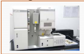
Leco carbon-sulfur analyzer
