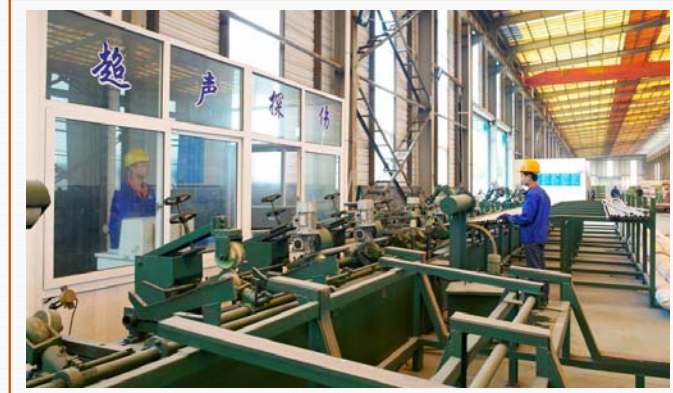
Ultrasonic Flaw Detection (UT)
