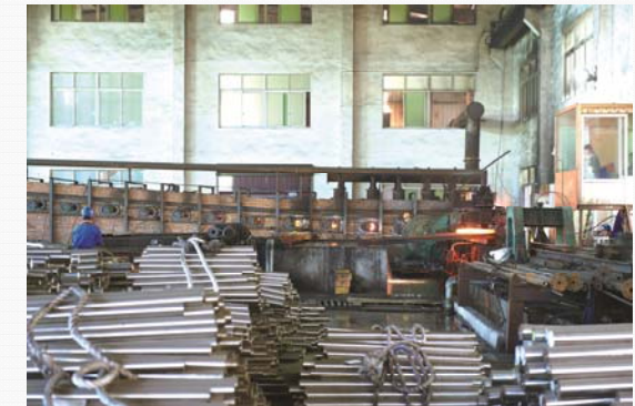
4 Automatic hot Piercing production line
