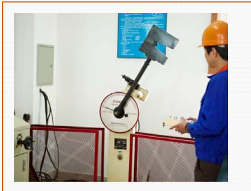
Impact testing machine
