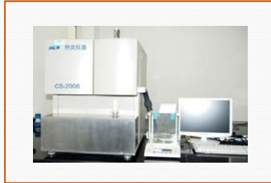
NCS carbon-sulfur analyzer
